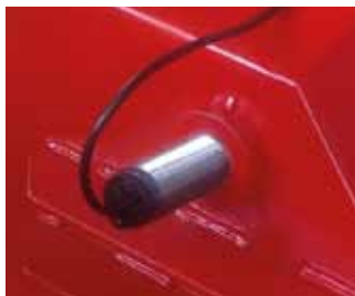
Speed / Rotational Sensor To confirm correct operation of the exciter
